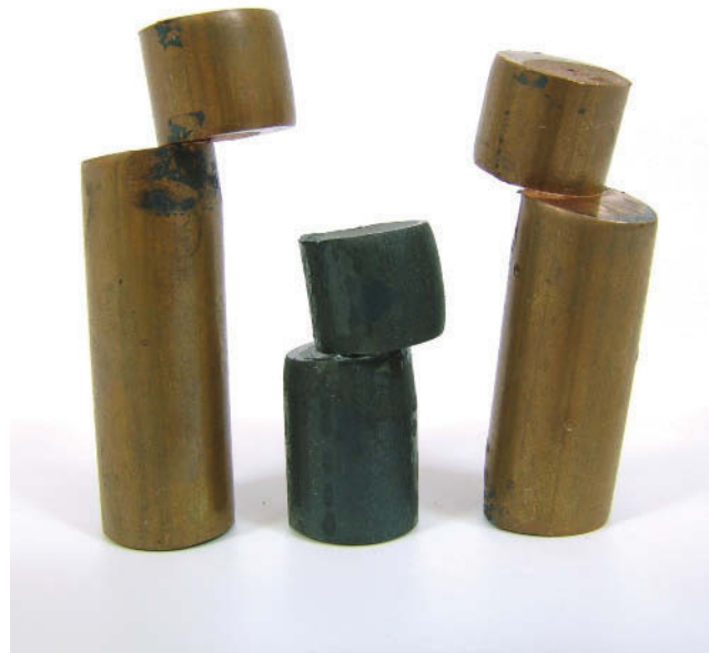
FIGURE 1.3 Single-shear failure in pin specimens.
