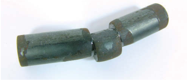
FIGURE 1.4 Double-shear failure in a pin specimen.
